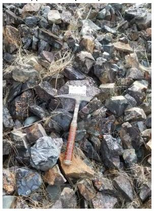
Figure 3-25 Photographs of slag fragments from the dump (note photograph on left shows copper oxide staining) ( SRK ES Sept 2019)
