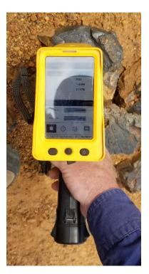
Figure 3-24 Using pXRF to verify the grade range of slag fragments from the dump (left to right; 954ppm As, 6,180ppm Cu, 3.013% Zn; 925ppm As, 6,210ppm Cu, 3.035% Zn; and 1,832ppm As, 1.938% Cu, 2.107% Zn) ( SRK ES Sept 2019)
