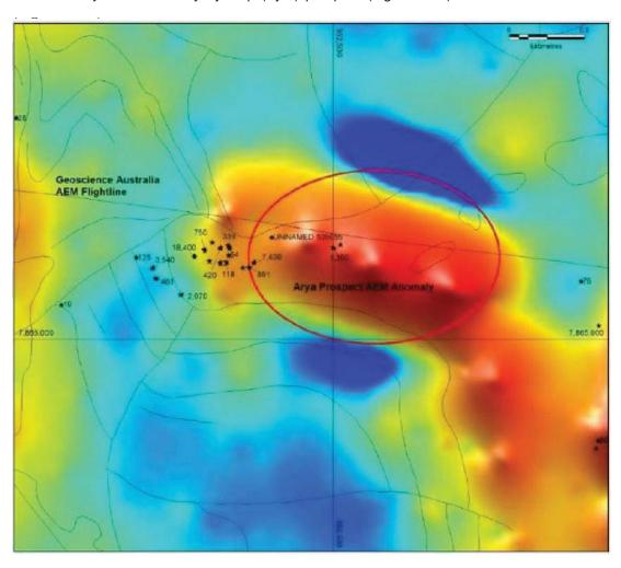
Figure 5-11 – Airborne magnetic response over the Ayra prospect. Samples labelled by copper assay results (Source: SRK Competent Person's Report)
