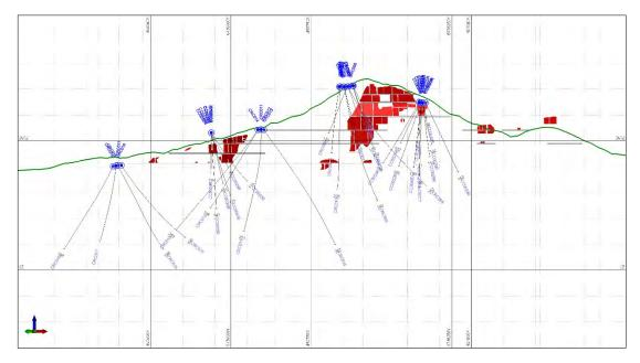
Figure 3-18 Cangai Mine longitudinal section, showing location and trace of RC holes drilled by Castillo Copper, red blocks are modelled Resource blocks (Image Source: Castillo Copper Micromine Model, 2018)
