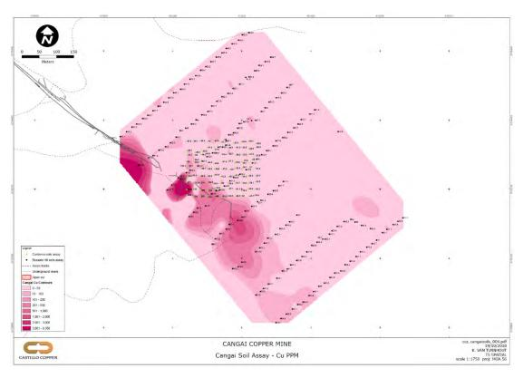
Figure 3-17 Contoured copper in soil results from Castillo's July & September 2018 soil sampling programmes (Image Source: T5 Spatial, 2018)
