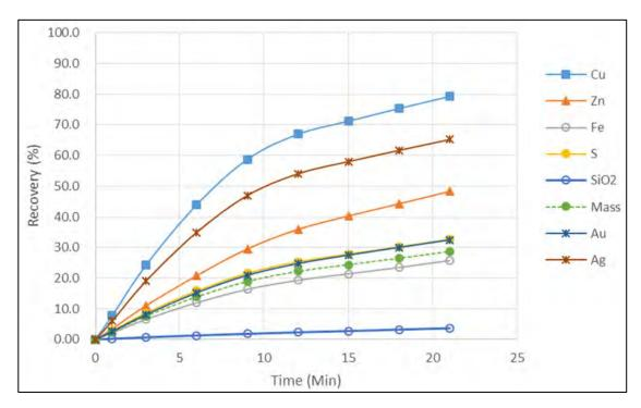
Figure 3-21 Graph to show Cangai Massive Sulphide Composite Flotation Kinetics P<sub>80</sub> 53μm with 15μm Regrind RDA2805 (Source: ALS Metallurgy, 2020)
