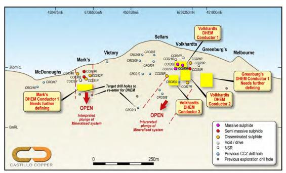
Figure 3-16 DHEM conductors at the Cangai Mine (Image Source: Castillo Copper, 2018c)
